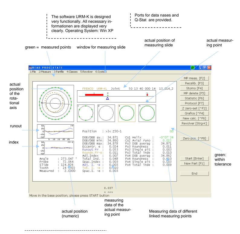
The FRENCO measuring electronic MEG 32 links the measuring instrument to the integrated PC.
